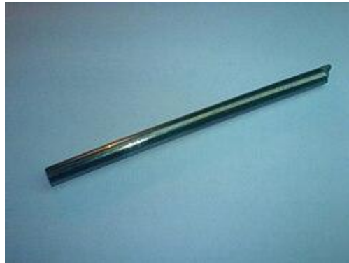
Figure 2. Single crystal of bismuth telluride [4]
