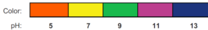
Fig. 4. Concrete discoloration chart for the control liquid - Rainbow Test (based on materials from Germann Instruments)
