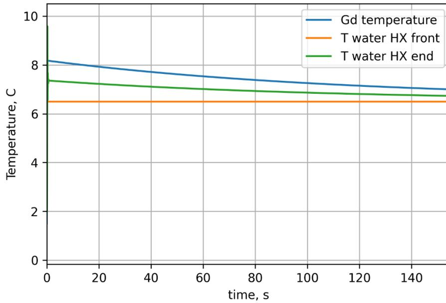
**Figure 11.** Temperature changes during the process of cooling Gadolinium by the chiller
