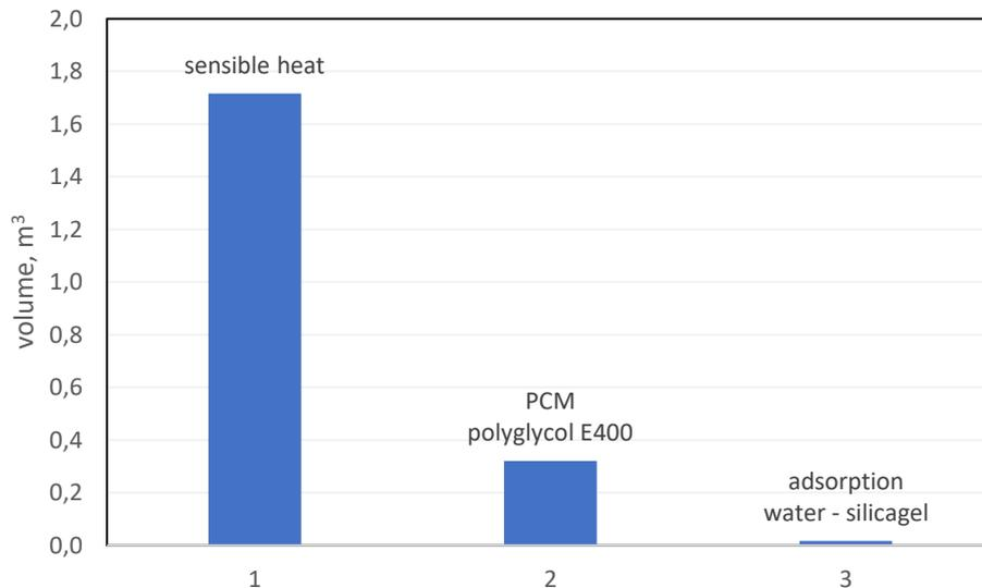
**Figure 1.** Comparison of cold storage methods for 10 kWh of cold
