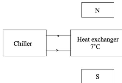
**Figure 7.** Cooling down heat exchanger material by chiller (under magnetic field)
