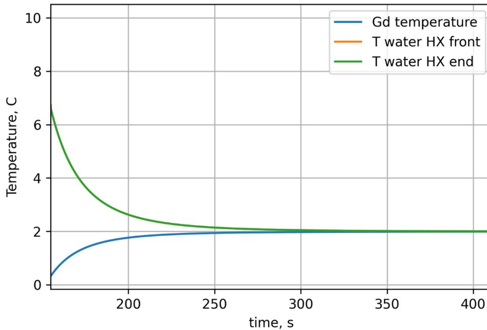
**Figure 12.** Temperature change during the process of equalizing temperature after a change in magnetic field intensity
