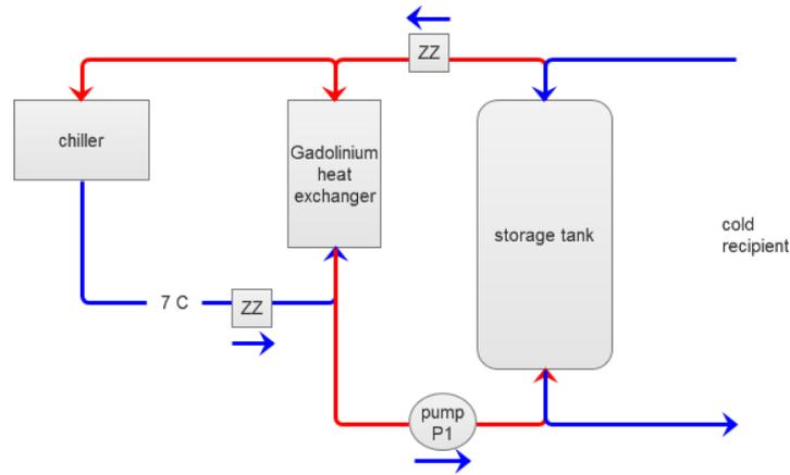
**Figure 4.** The analyzed cold storage system
