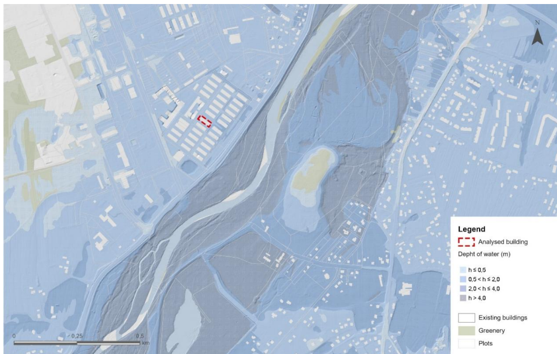
Fig. 3. Projected water height in case of failure, damage or destruction of damming structure (own study)
