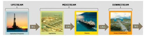
Figure 2. The supply chain of the LNG [5]
