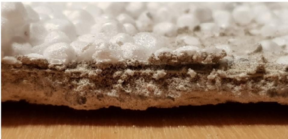
Figure 2. Details of thermal insulation (substrate) a), b) and c) for the ceramic cladding of the building facade
