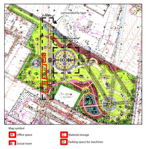
Figure 9. Diagram of the development of the construction site on the map [13]
