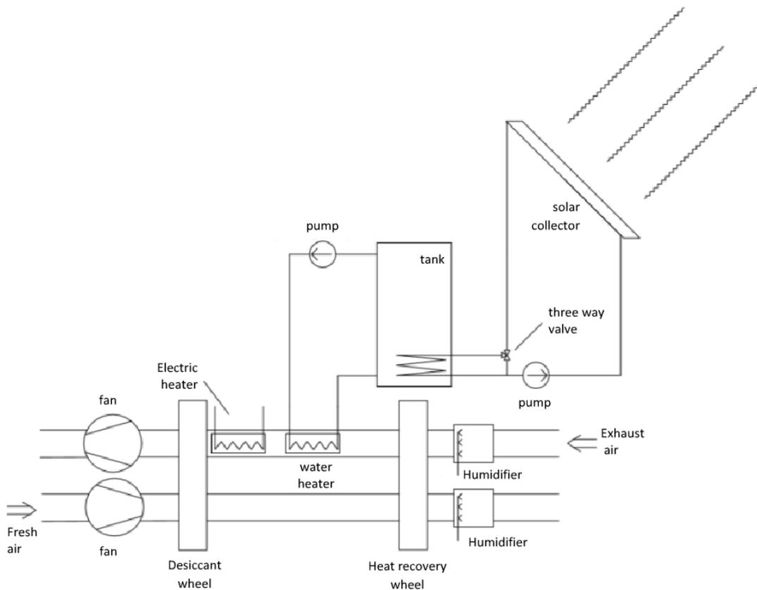
Figure 3. Analysed DEC system
