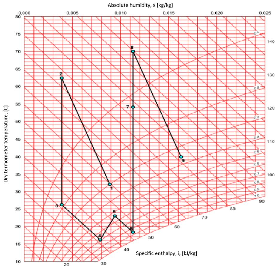
Figure 2. Thermodynamic changes of air taking place in a DEC type air handling unit
