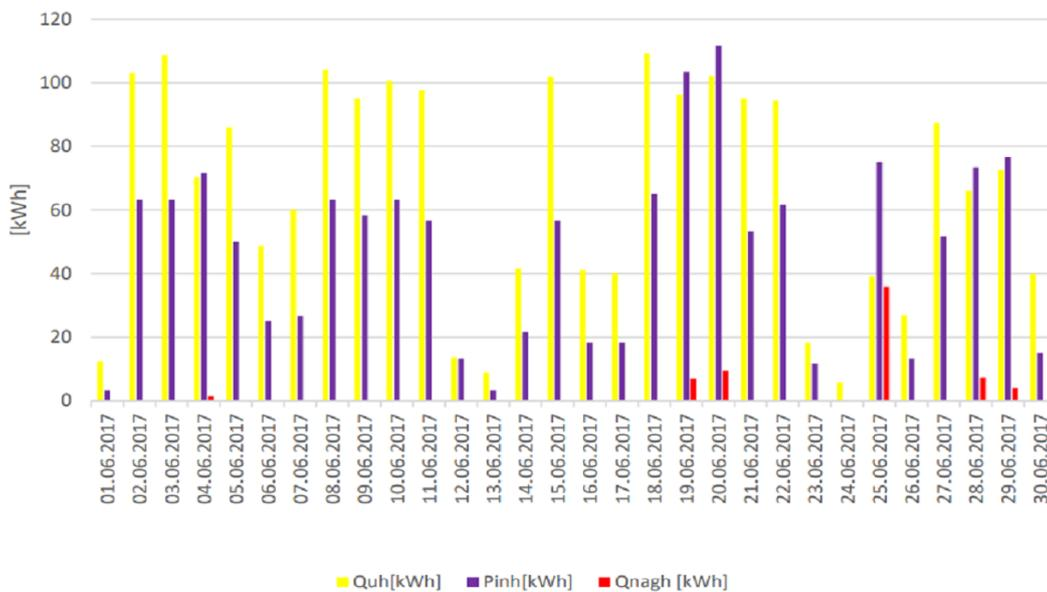
Figure 9. The amount of energy obtained in solar collectors, supplied to the electric heater and consumed by the DEC system in conditions corresponding to the days of June 2017.  $Q_{uh}$ - the amount of useful energy obtained in the collectors during the day,  $P_{inh}$  - the amount of energy supplied for the regeneration of the sorption rotor during the day,  $Q_{nagd}$  - the amount of energy supplied to the electric heater during the day.
