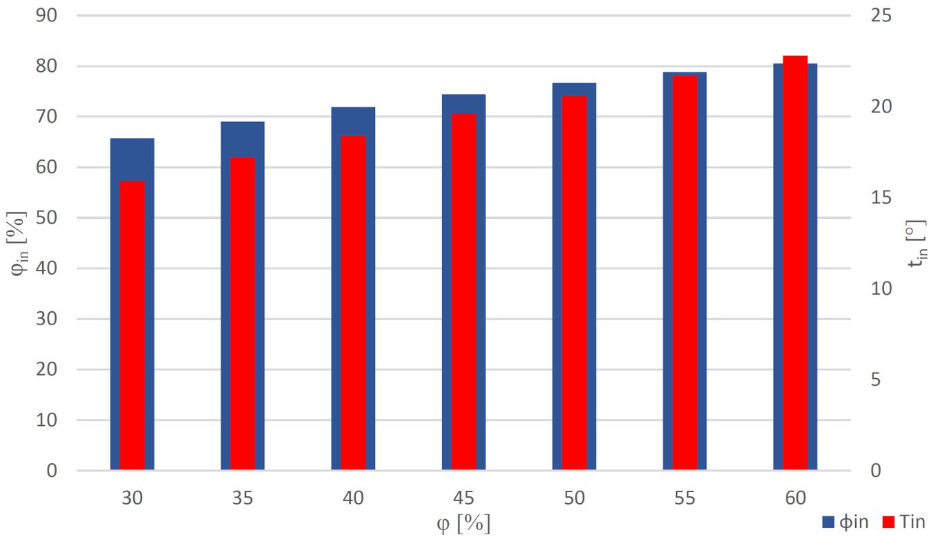
Figure 5. Influence of the relative humidity of the outside air  $\phi$  on the temperature  $t_{in}$  and the relative humidity  $\phi_{in}$  of the supply air to the rooms
