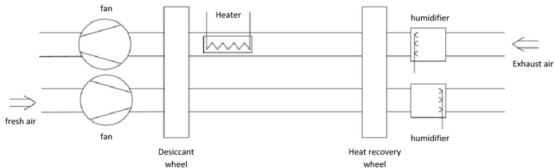
Figure 1. DEC system schema
