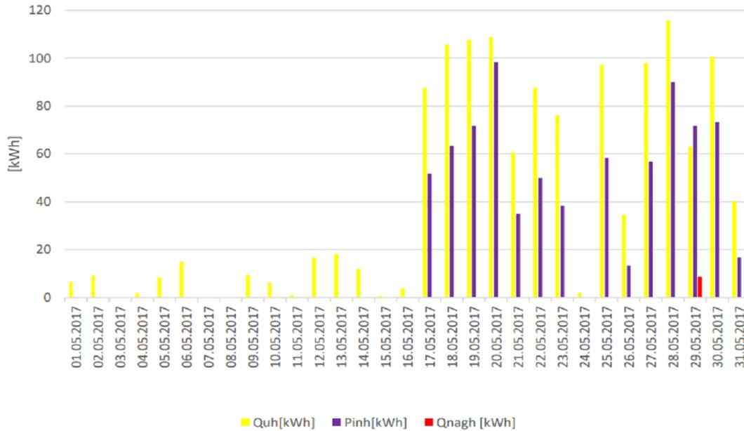
Figure 8. The amount of energy obtained in solar collectors, supplied to the electric heater and consumed by the DEC system in conditions corresponding to the days of May 2017.  $Q_{uh}$ - the amount of useful energy obtained in the collectors during the day,  $P_{inh}$  - the amount of energy supplied for the regeneration of the sorption rotor during the day,  $Q_{nagd}$  - the amount of energy supplied to the electric heater during the day.
