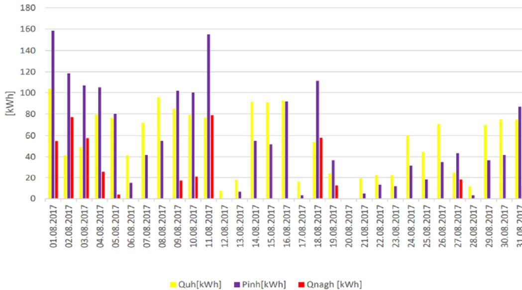
Figure 11. The amount of energy obtained in solar collectors, supplied to the electric heater and consumed by the DEC system in conditions corresponding to the days of August 2017.  $Q_{uh}$ - the amount of useful energy obtained in the collectors during the day,  $P_{inh}$  - the amount of energy supplied for the regeneration of the sorption rotor during the day,  $Q_{nagd}$  - the amount of energy supplied to the electric heater during the day.
