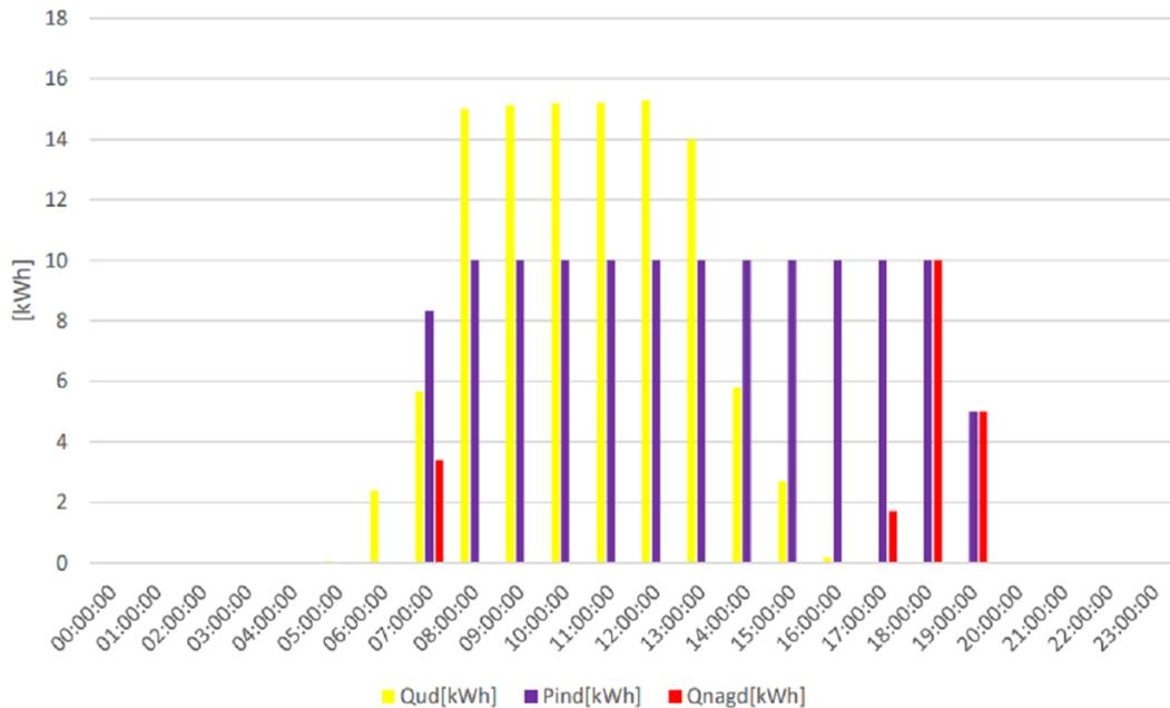
Figure 12. The amount of energy obtained in solar collectors, supplied to the electric heater and consumed by the DEC system in conditions corresponding to the next hours of 30.07.2017.  $Q_{ud}$  - the amount of useful energy obtained in the collectors in an hour,  $P_{ind}$  - the amount of energy supplied for the regeneration of the sorption rotor in an hour,  $Q_{nagd}$  - the amount of energy supplied to the electric heater in an hour.
