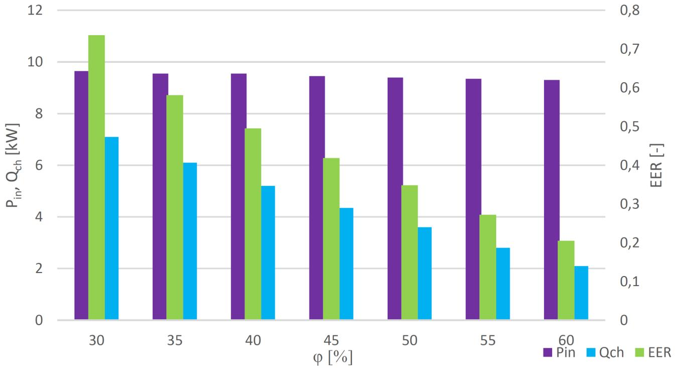
Figure 4. The influence of the relative humidity of the outside air  $\phi$  on the cooling power  $Q_{ch}$ , the power supplied for the regeneration  $P_{in}$  and EER for analysed DEC system
