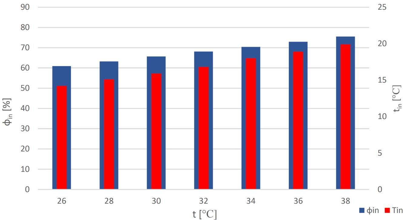
Figure 7. Influence of outdoor air temperature  $t$  on temperature  $t_{in}$  and relative humidity  $\phi_{in}$  of room air
