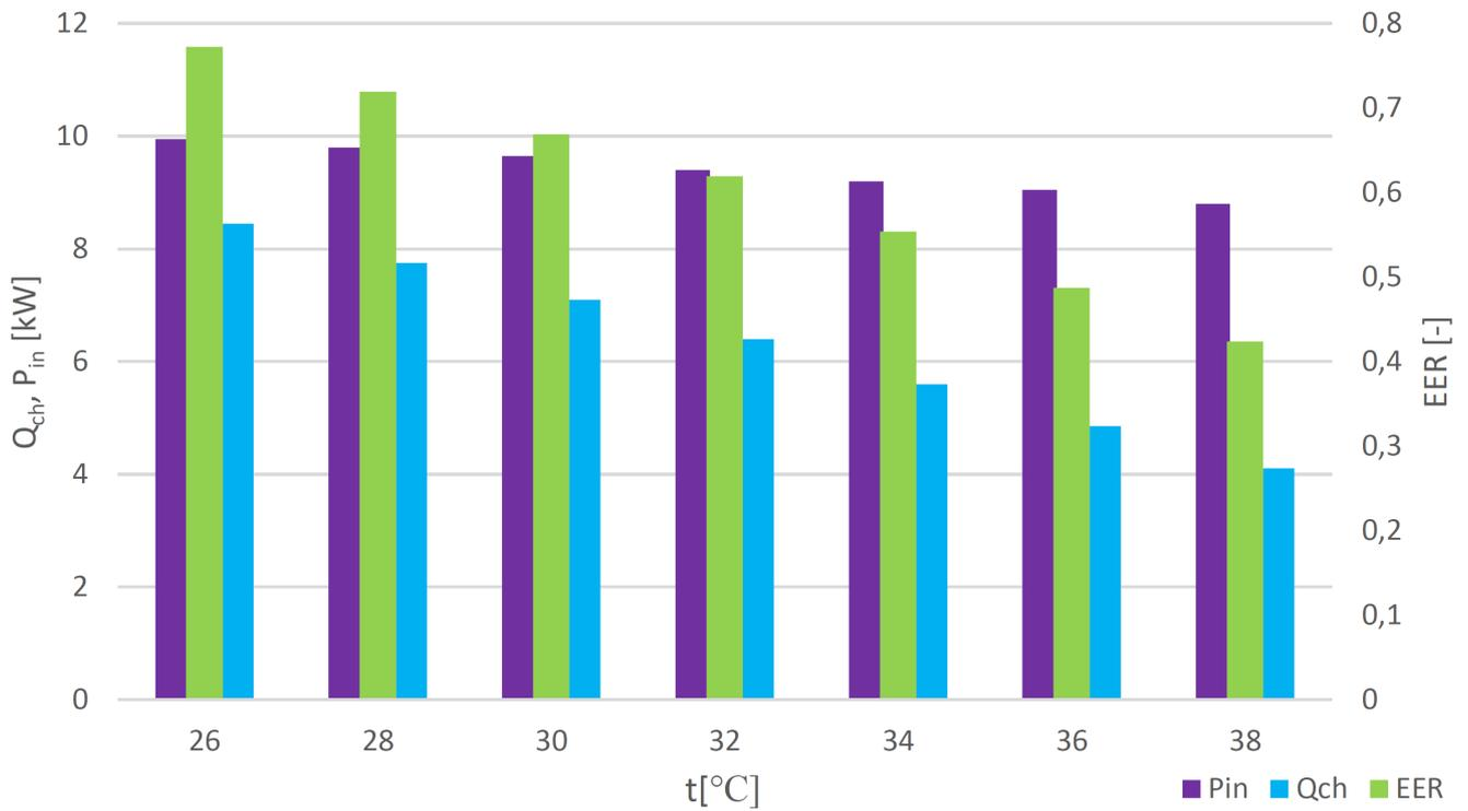
Figure 6. Influence of outside air temperature  $t$  on  $Q_{ch}$  cooling power, power supplied for regeneration of the  $P_{in}$  and EER of sorption rotor for analysed DEC system
