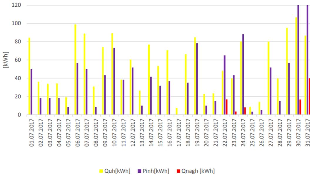
Figure 10. The amount of energy obtained in solar collectors, supplied to the electric heater and consumed by the DEC system in conditions corresponding to the days of July 2017.  $Q_{uh}$ - the amount of useful energy obtained in the collectors during the day,  $P_{inh}$  - the amount of energy supplied for the regeneration of the sorption rotor during the day,  $Q_{nagd}$  - the amount of energy supplied to the electric heater during the day.
