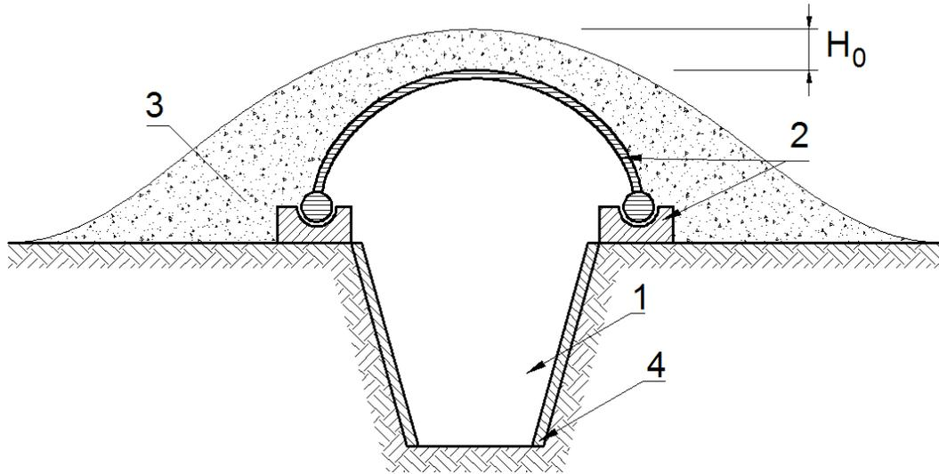
Figure 2. Example of a concealment solution, 1-trench or shooting ditch, 2-elements of laminate covering, 3- ground backfilling, H o-minimum thickness of the backfill, 4-covering of trench slopes frommaters or laminates
