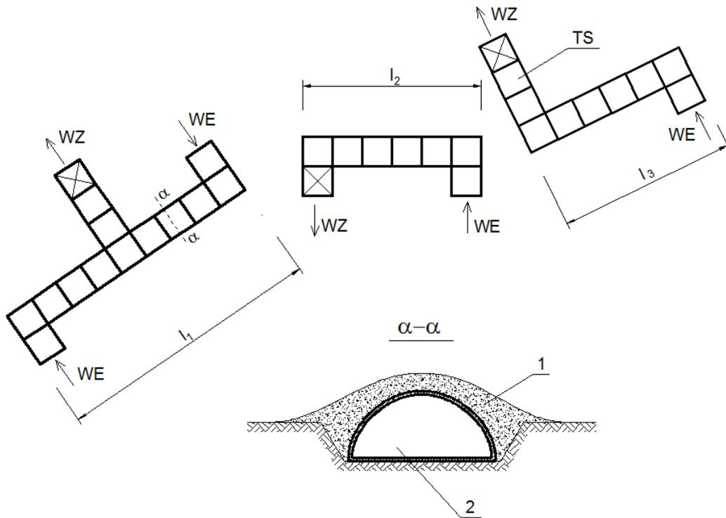
Figure 3. Diagram of possible location of temporary hides in the field, TS-typical modol,  $l_1$ ,  $l_2$ ,  $l_3$ - length of single hides, WZ, WE-closing elements, 1-back, 2-cross-section of a typical module
