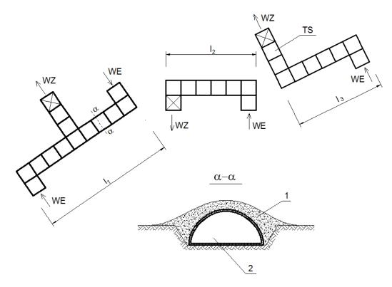
Figure 3. Diagram of possible location of temporary hides in the field, TS-typical modol,  $l_1$ ,  $l_2$ ,  $l_3$ - length of single hides, WZ, WE-closing elements, 1-back, 2-cross-section of a typical module
