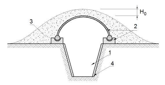
Figure 2. Example of a concealment solution, 1-trench or shooting ditch, 2-elements of laminate covering, 3- ground backfilling, H o-minimum thickness of the backfill, 4-covering of trench slopes frommaters or laminates
