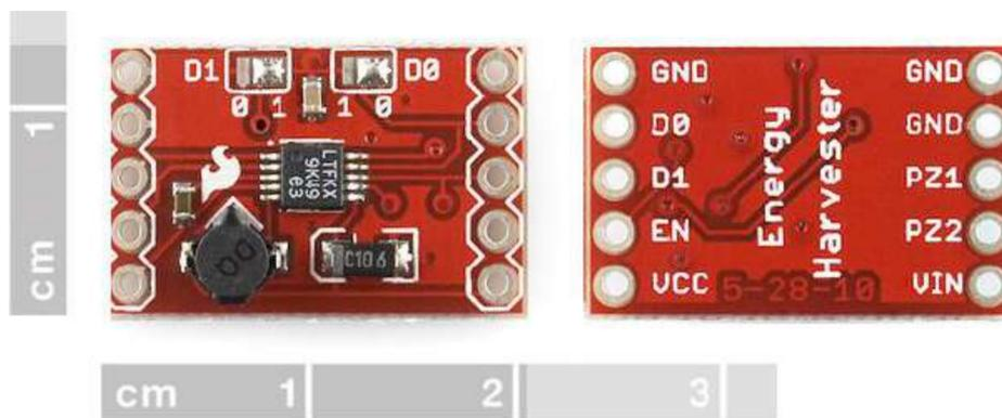
Figure 1. Piezoelectric Energy Harvesting Power Supply
