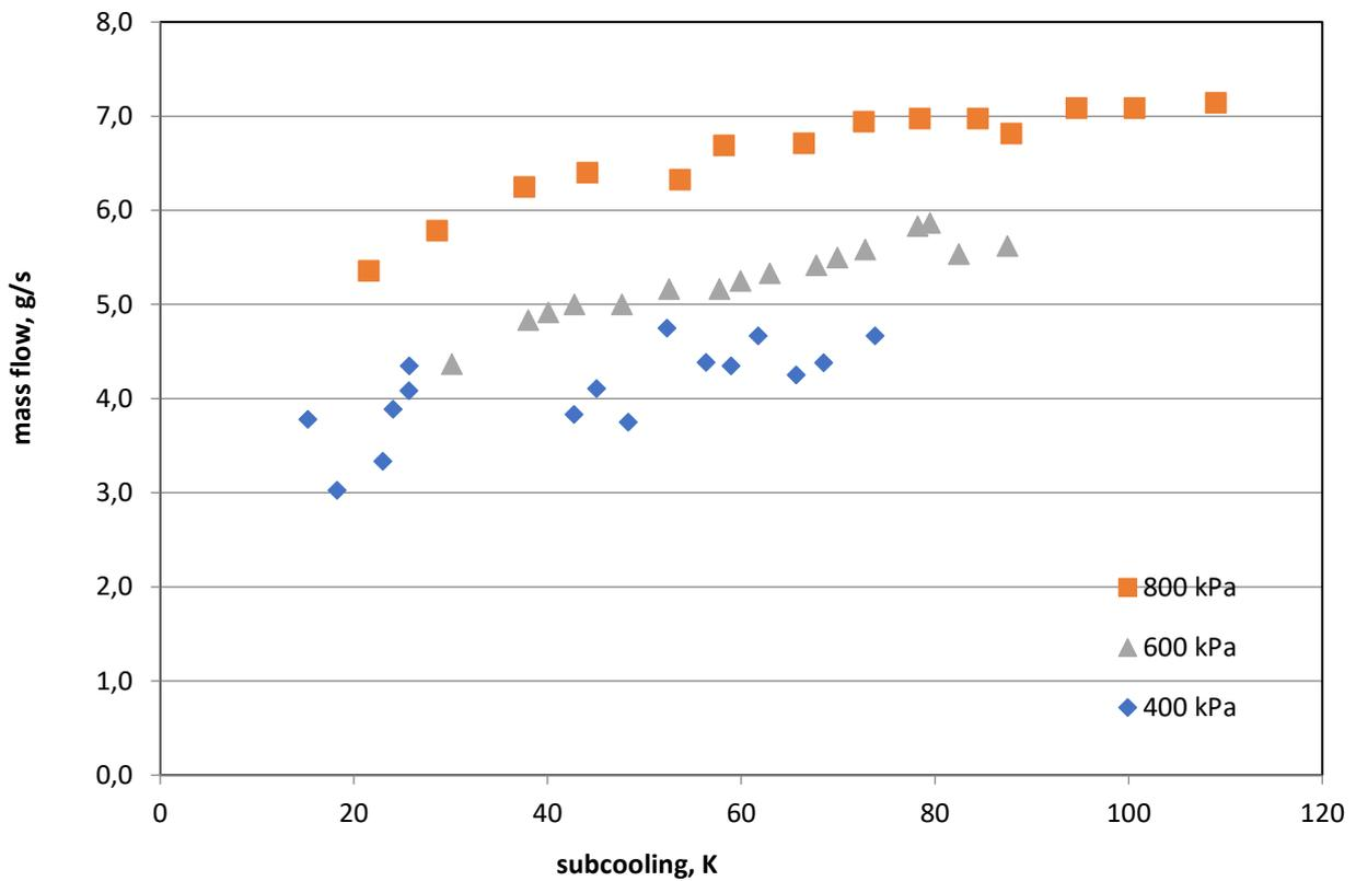
Figure 8. Mass flow of condensate as a function of subcooling value for a steam trap (nozzle diameter  $D=0.60$  mm)
