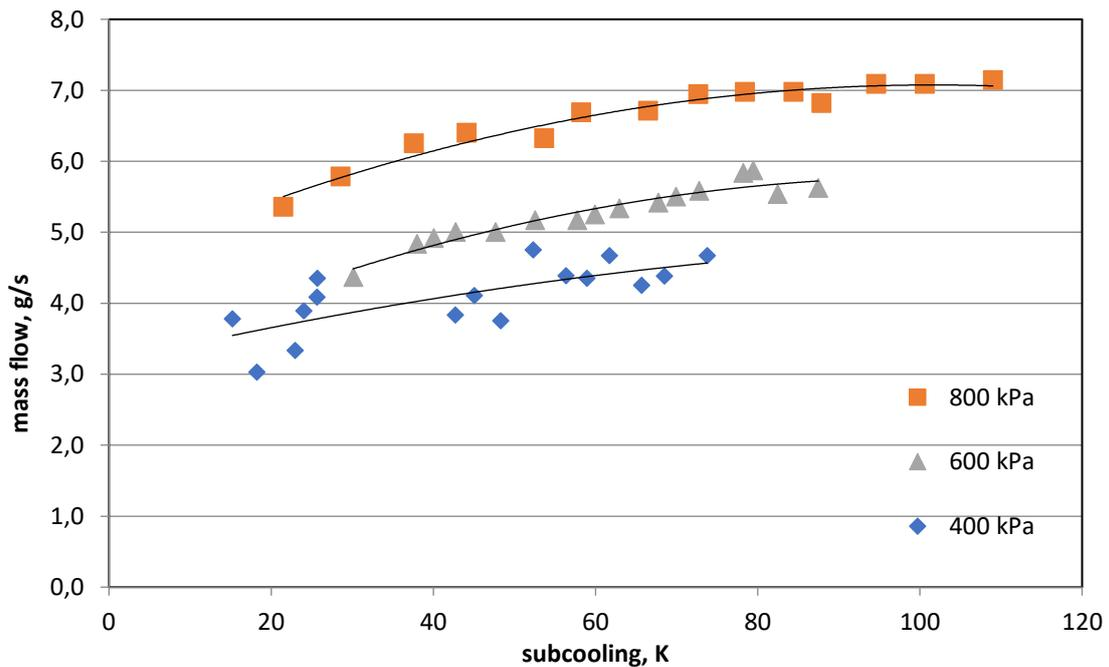
Figure 13. Approximation of operating characteristics of steam traps with nozzle diameter D=0.60mm
