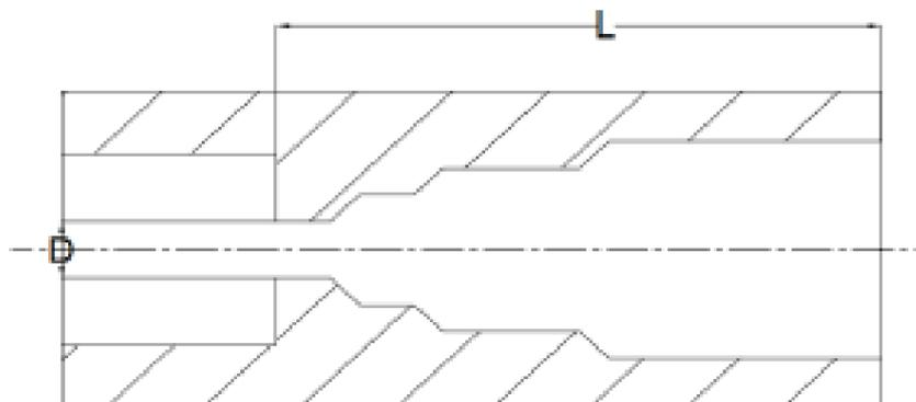
Figure 5. Cross-section of the examined steam traps
