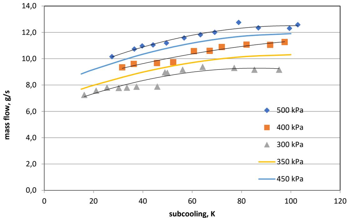
Figure 20. Determined operating characteristics of the steam trap for pressures level equal to 350 and 450 kPa, stem trap with nozzle diameter  $D=0.97\text{mm}$
