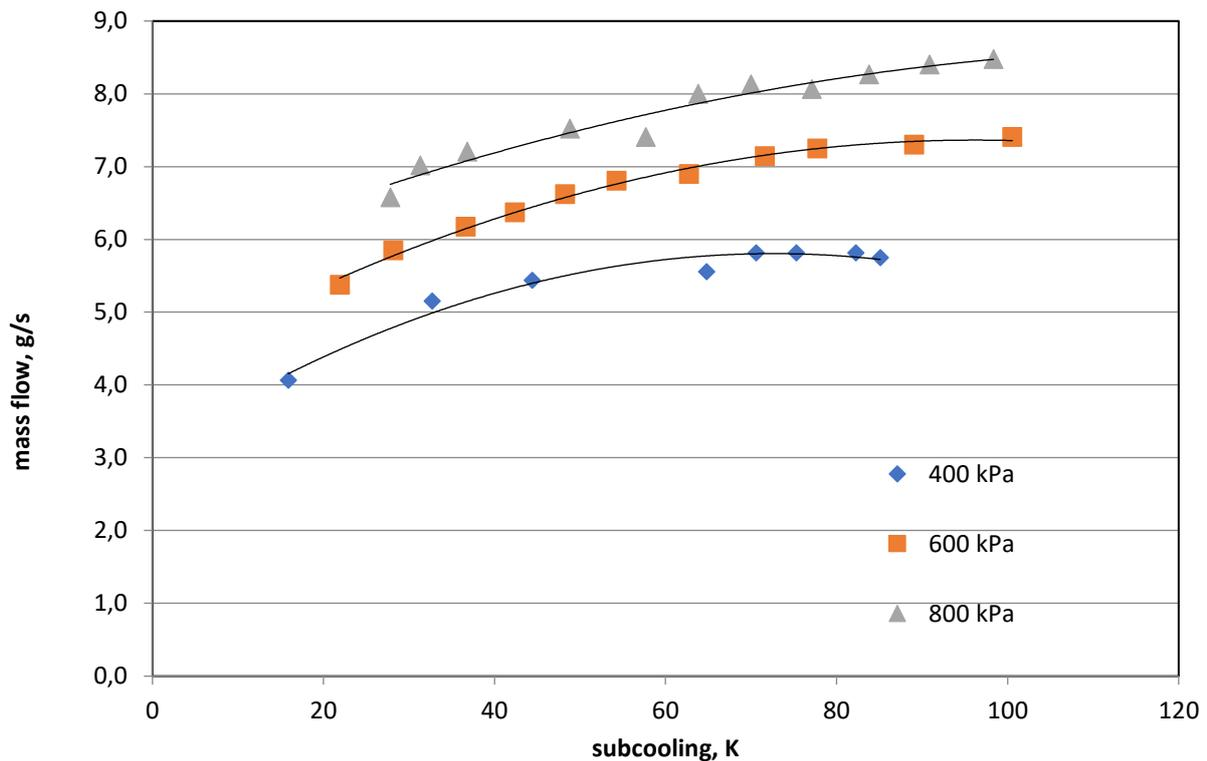
Figure 14. Approximation of operating characteristics of steam traps with nozzle diameter D=0.67mm
