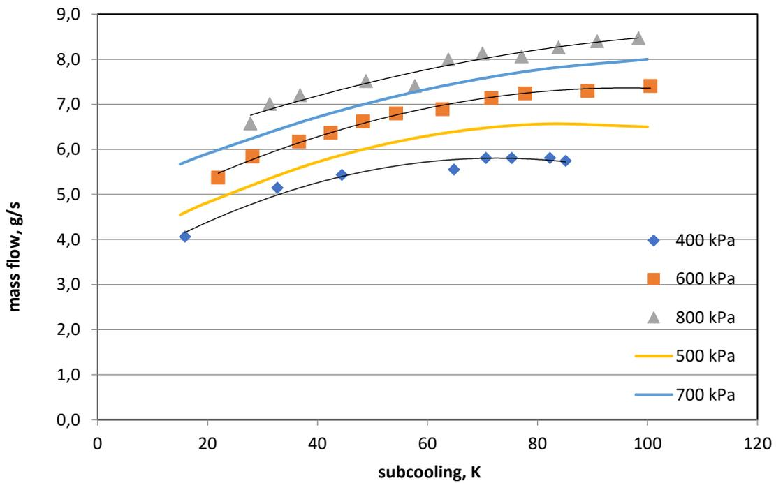
Figure 19. Determined operating characteristics of the steam trap for pressures level equal to 500 and 700 kPa, stem trap with nozzle diameter  $D=0.67\text{mm}$
