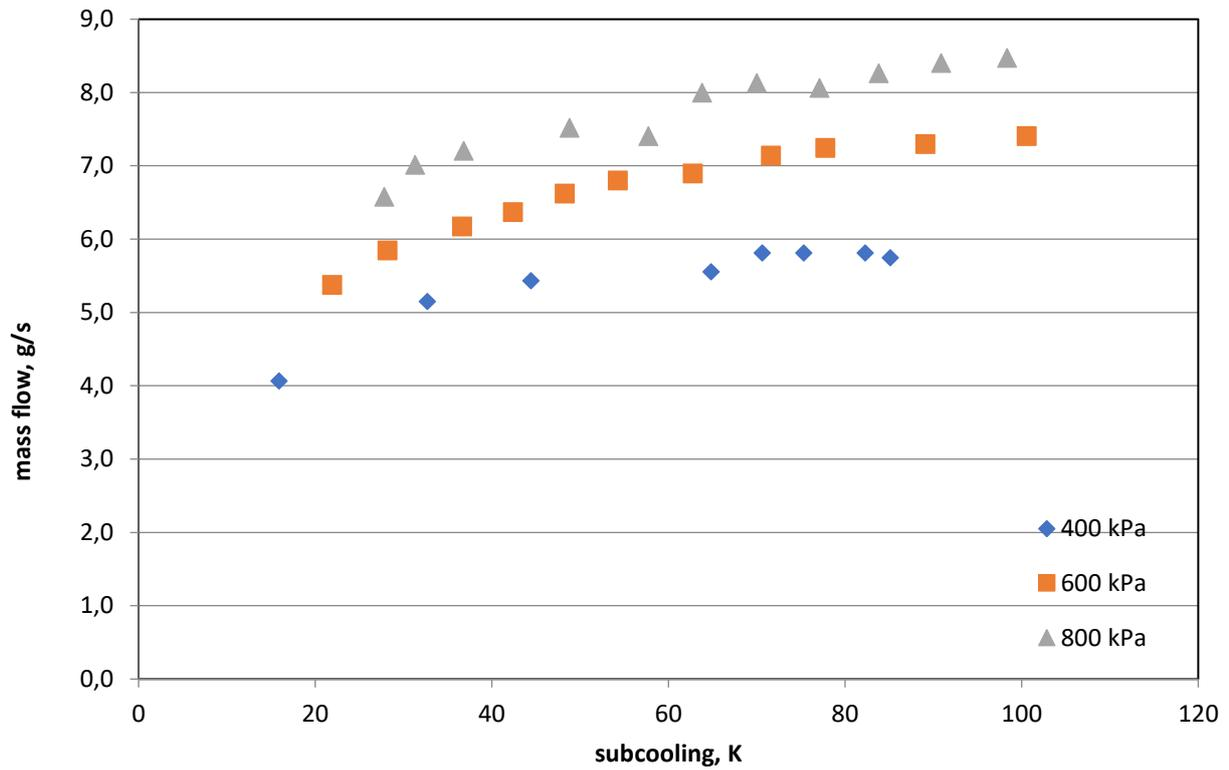
Figure 9. Mass flow of condensate as a function of subcooling value for a steam trap (nozzle diameter  $D=0.67$  mm)
