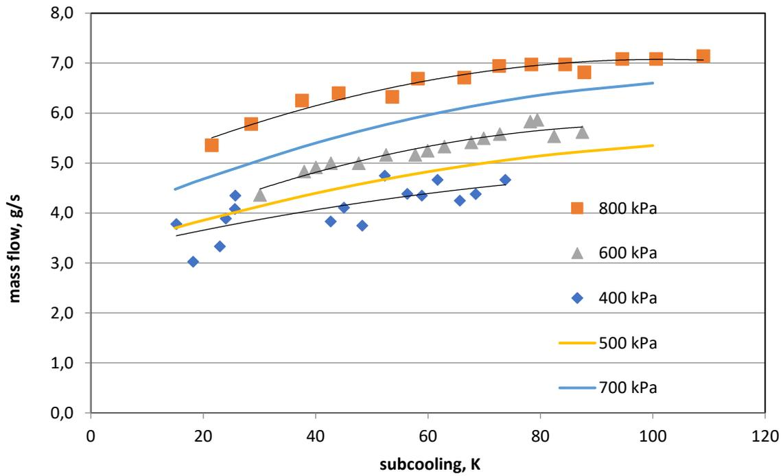
Figure 18. Determined operating characteristics of the steam trap for pressures level equal to 500 and 700 kPa, stem trap with nozzle diameter  $D=0.60\text{mm}$
