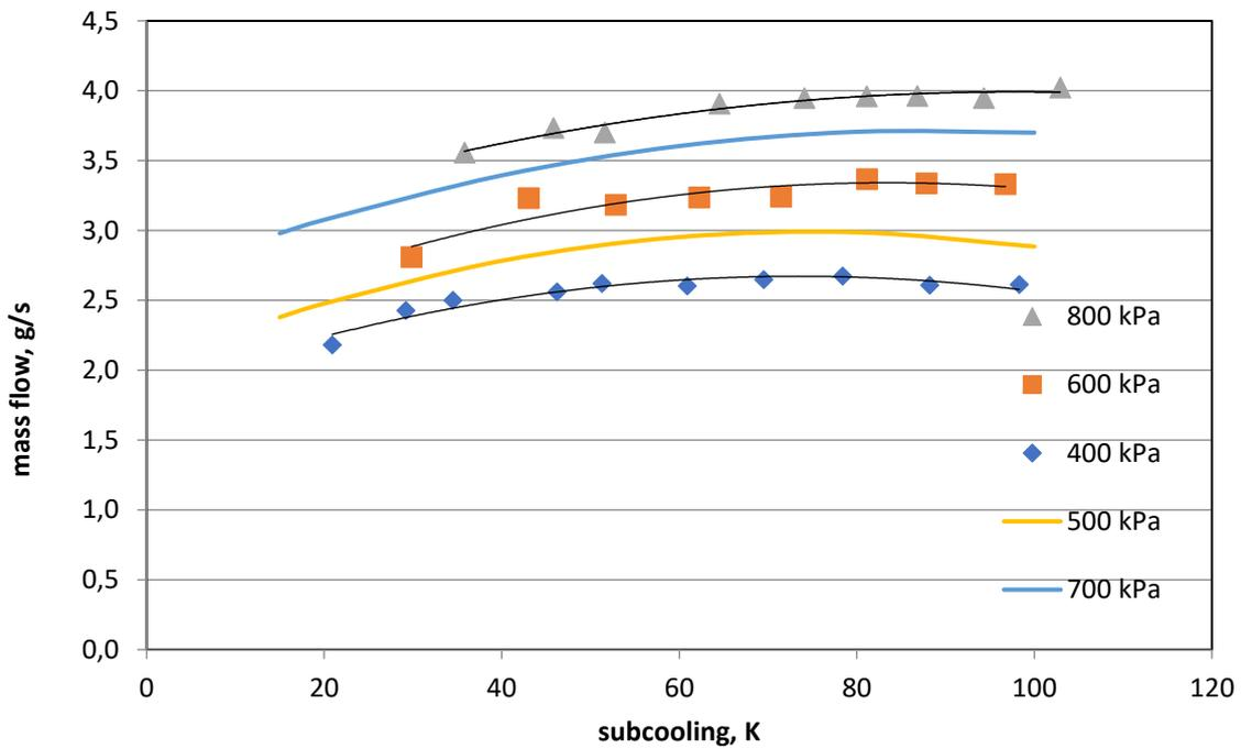
Figure 17. Determined operating characteristics of the steam trap for pressures level equal to 500 and 700 kPa, stem trap with nozzle diameter  $D=0.51\text{mm}$
