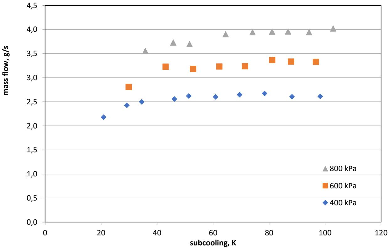
Figure 7. Mass flow of condensate as a function of subcooling value for a steam trap (nozzle diameter  $D=0.51$  mm)
