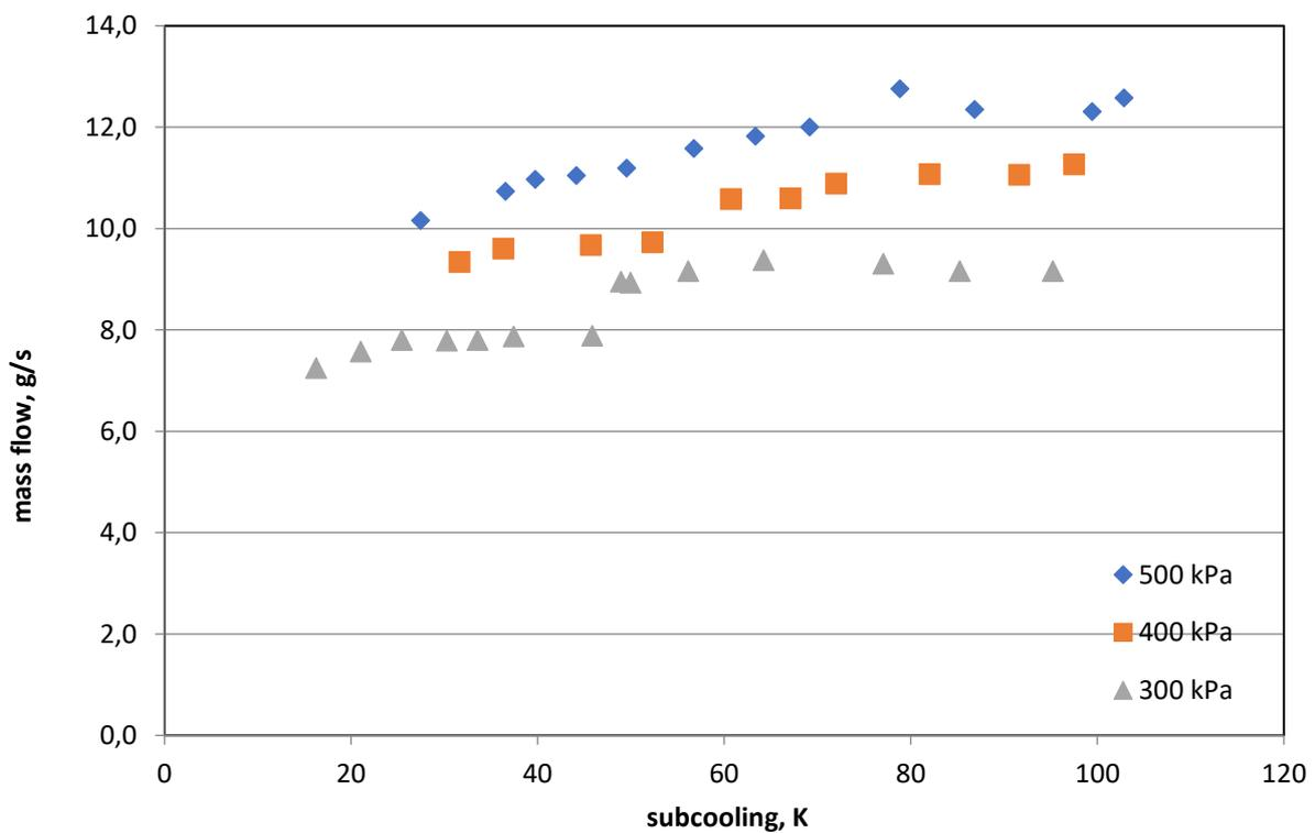
Figure 10. Mass flow of condensate as a function of subcooling value for a steam trap (nozzle diameter  $D=0.97$  mm)
