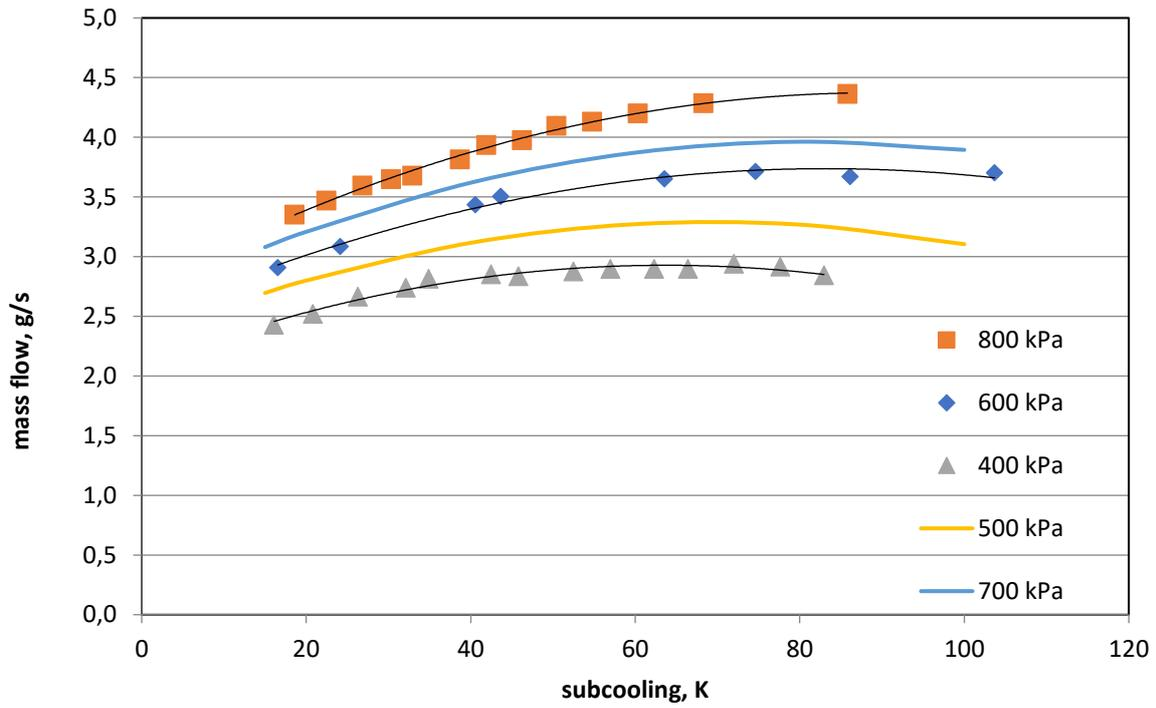
Figure 16. Determined operating characteristics of the steam trap for pressures level equal to 500 and 700 kPa, stem trap with nozzle diameter  $D=0.47\text{mm}$
