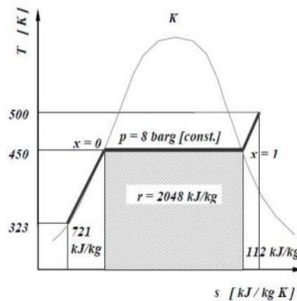
Figure 1. The amount of energy involved in the phase change process for steam [24].
