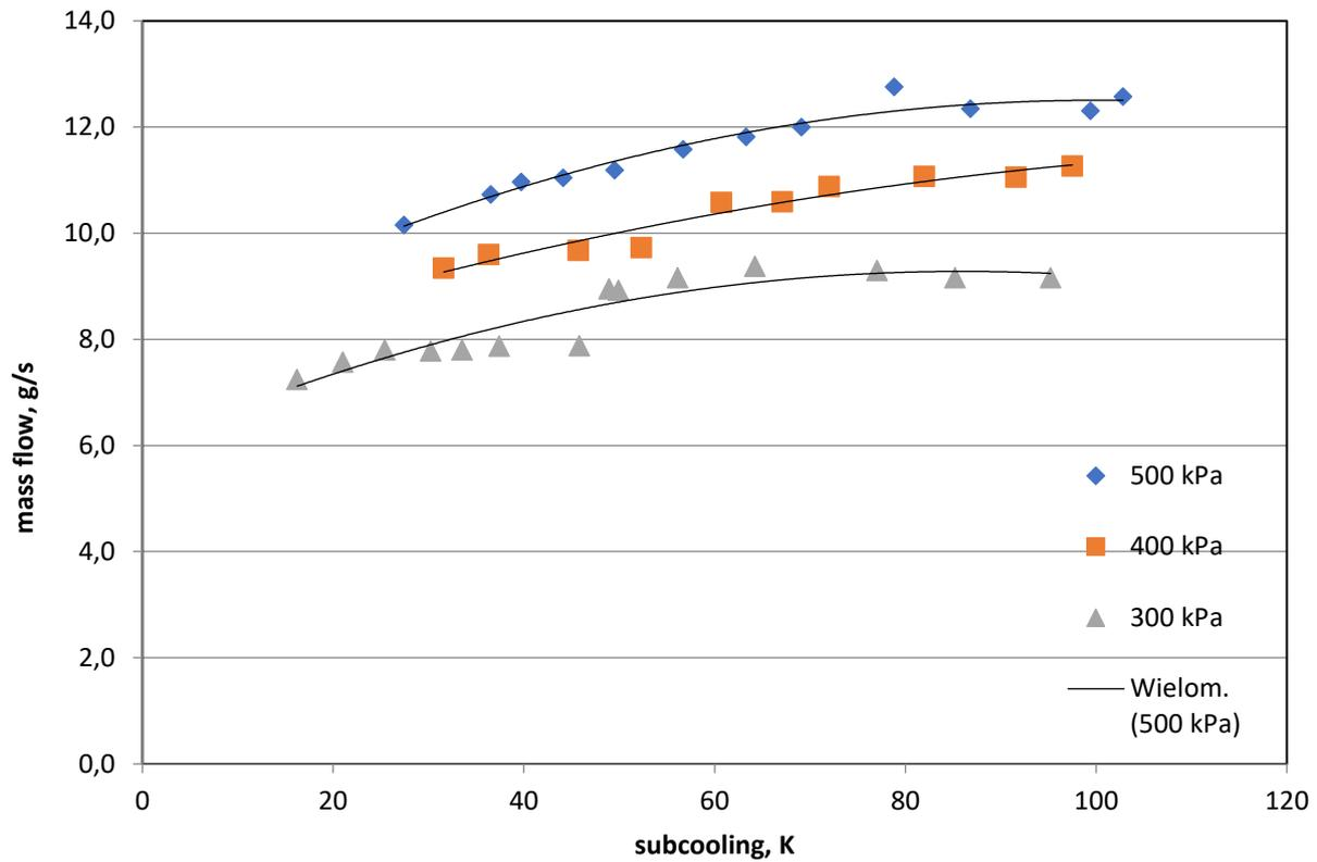
Figure 15. Approximation of operating characteristics of steam traps with nozzle diameter  $D=0.97\text{mm}$
