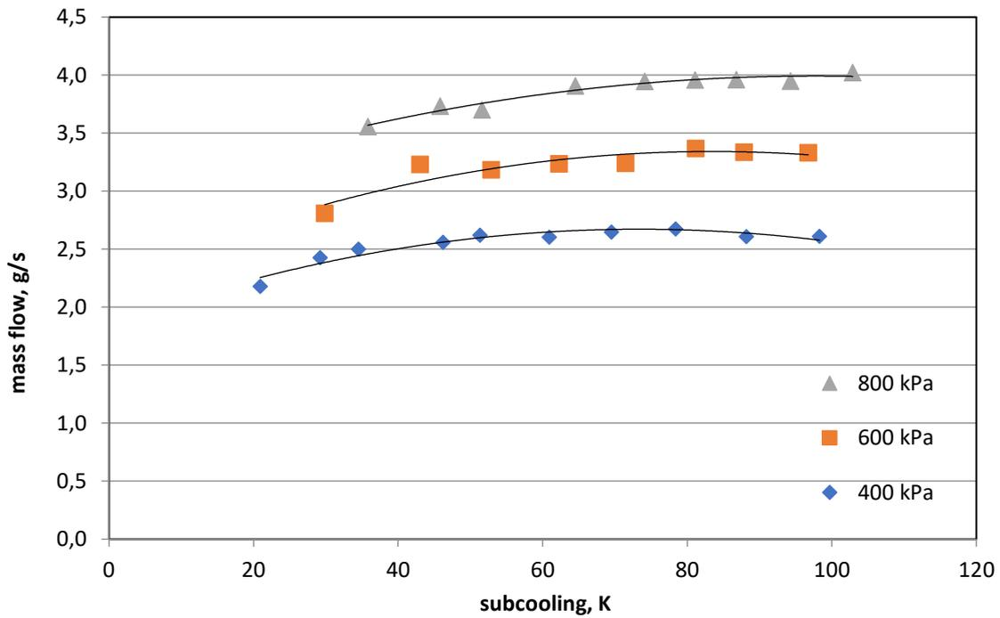
Figure 12. Approximation of operating characteristics of steam traps with nozzle diameter D=0.51mm
