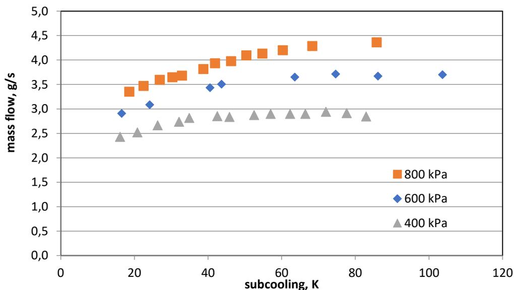
Figure 6. Mass flow of condensate as a function of subcooling value for a steam trap (nozzle diameter D=0.47 mm)
