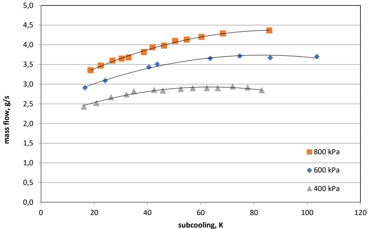
Figure 11. Approximation of operating characteristics of steam traps with nozzle diameter  $D=0.47\text{mm}$
