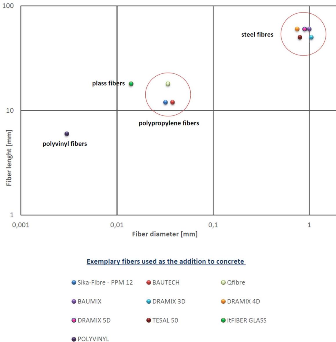
Figure 1. The dimensions of fibers used as the addition to the cement concrete
